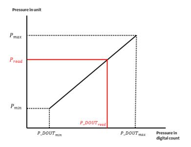
For example, the  $P_{min}$  and  $P_{max}$  for the sensor are specified as -10cmH<sub>2</sub>O and +10cmH<sub>2</sub>O. The  $DOUT_{min}$  and  $DOUT_{max}$  are -26214 and +26214. So,
